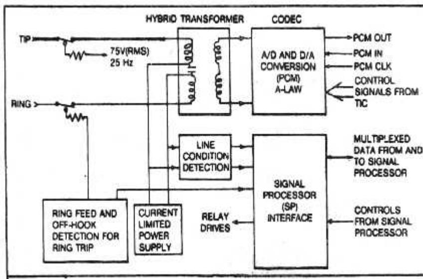
Fig 8.1 Functional block diagram of Subscriber Line circuit card
