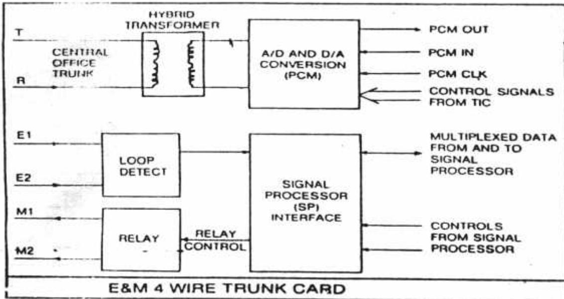
**Fig.9.2. Block diagram of E&M 4 wire trunk card.**
