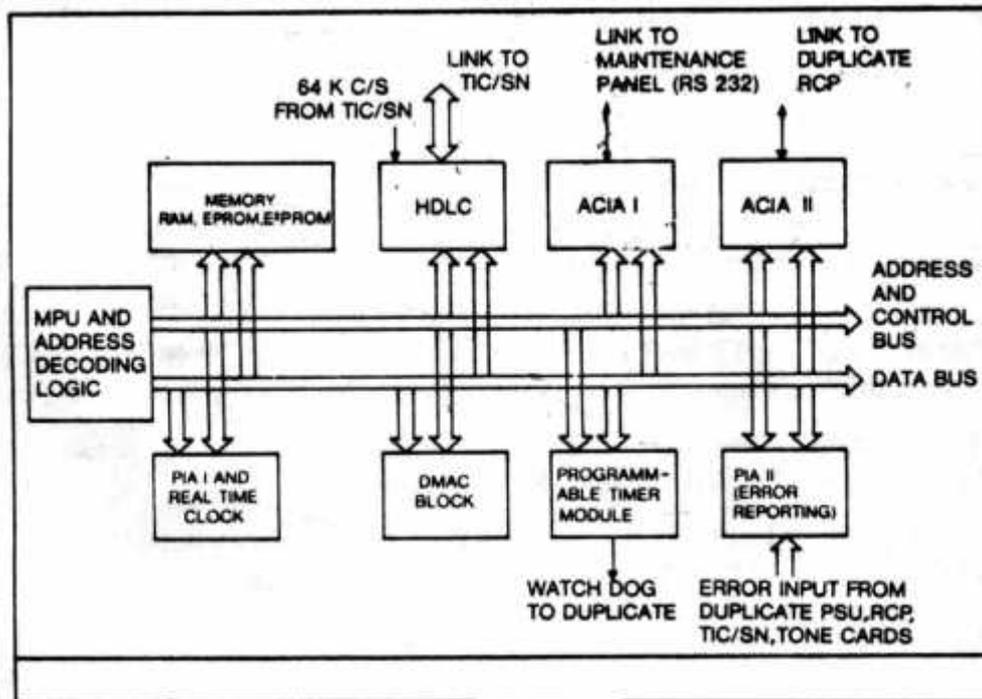
Fig.3.1. Functional Block diagram of RCP card
