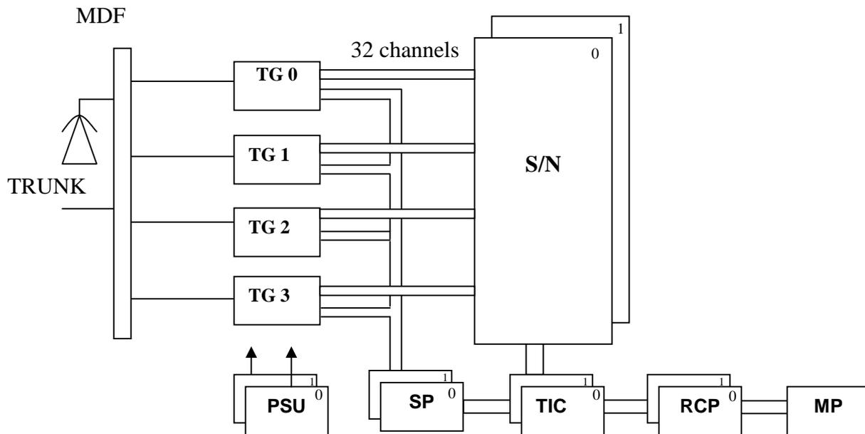
Fig 1.1 – System Architecture of C- DOT 128 Port RAX
